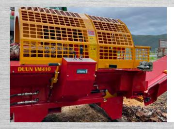
Joystick ensure operation of feeding, cutting, and splitting. Easy access to operation of hydraulic log holder.
