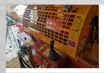
Joystick operation of feeding, cutting, and splitting. Operation of log holder and hatches that let the wood down into the splitting cradle by buttons on joystick. Adjustable speed and force on saw bar. Hydraulic side adjustment of discharge belt. Seamles
