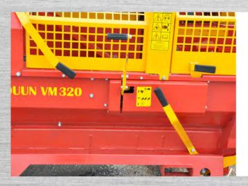
Operation of feeding belt, cutting cycle and splitting cycle in one multifunction lever.
