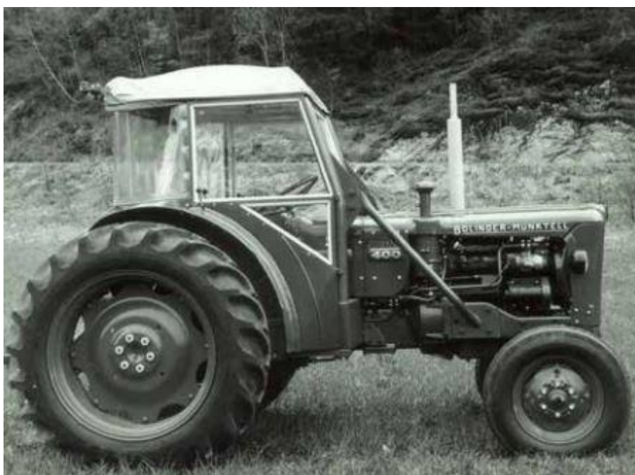
Winter-ready: Fully enclosed Duun protective arch for BM 400 Buster. This tractor model became important in the 1960s.
