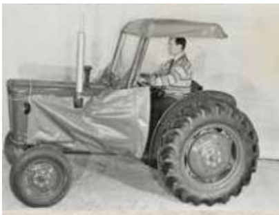
Driver protection: The earliest version of the Duun protective arch could be supplied with a fabric roof. Note the winter draft on the engine, which directed hot air backwards.
